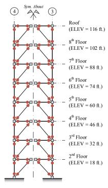
All columns, braces, and beams adjacent to link beams are force-controlled (FC) for flexure
