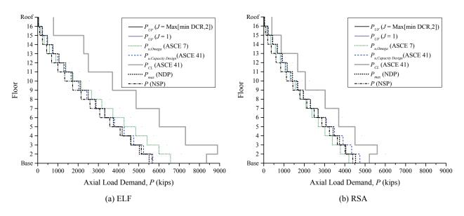
Figure 3-89. LDP Assessment Results, Compression in Exterior Columns, 16-Story EBF, BSE-1
