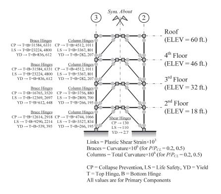
Figure 3-17. Frame Capacity Schematic (Inelastic), LS and CP, 4-Story EBF – ELF
