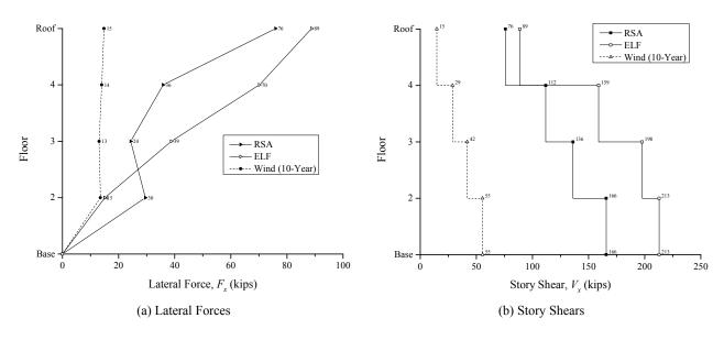
Figure B-2. Drift Design Lateral Forces and Story Shears
