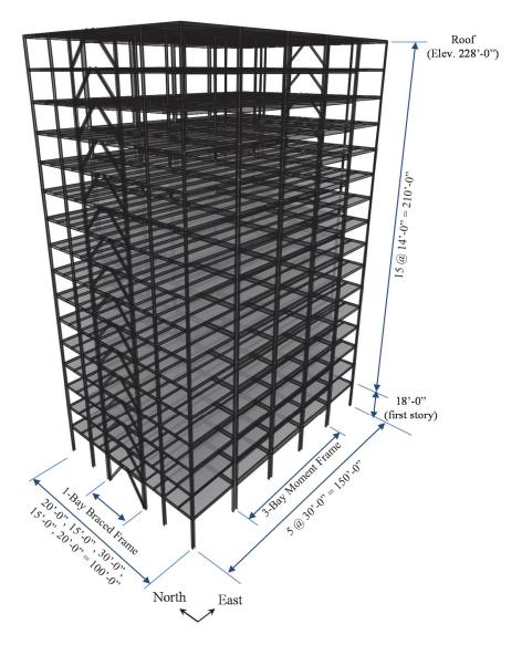
Figure 2-3. Isometric View of ME16 Archetype Building
