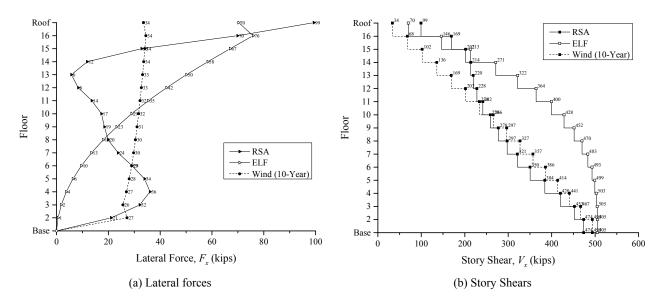
Figure B-17. Drift Design Lateral Forces and Story Shears
