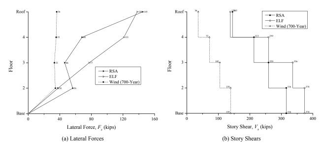
Figure B-1. Strength Design Lateral Forces and Story Shears
