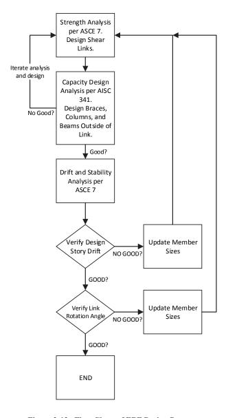
Figure 2-13. Flow Chart of EBF Design Process
