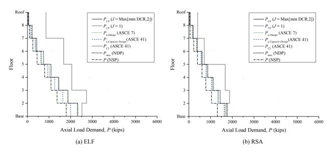
Figure 3-63. LDP Assessment Results, Compression in Exterior Columns, 8-Story EBF, BSE-2
