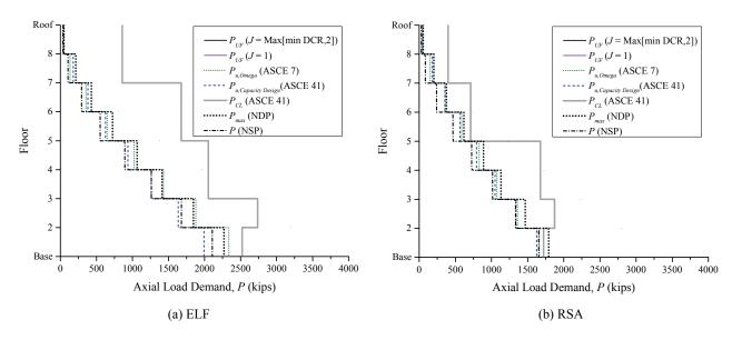
Figure 3-60. LDP Assessment Results, Compression in Exterior Columns, 8-Story EBF, BSE-1
