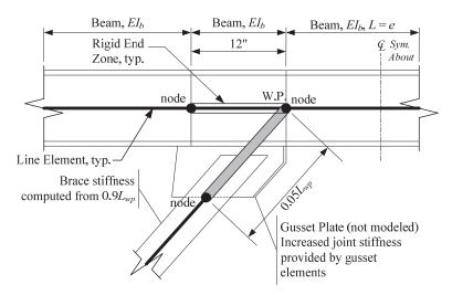
Figure 2-8. Brace-to-Beam Connection Subassembly Model for Linear Analysis
