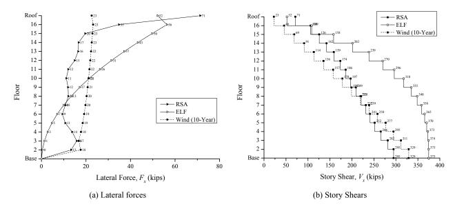
Figure B-8. Drift Design Lateral Forces and Story Shears
