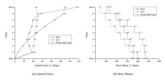
Figure B-4. Strength Design Lateral Forces and Story Shears
