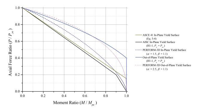
Figure 3-15. P-M Interaction Curve (Section Yield Surface)
