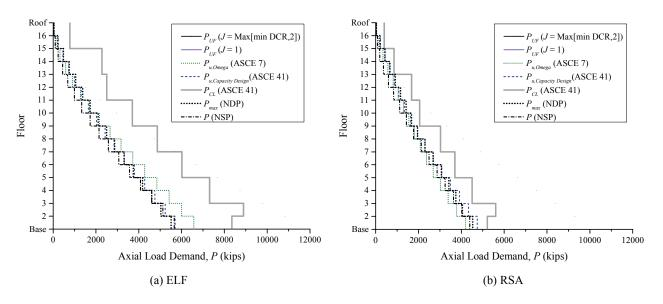
Figure 3-83. LSP Assessment Results, Compression in Exterior Columns, 16-Story EBF, BSE-1
