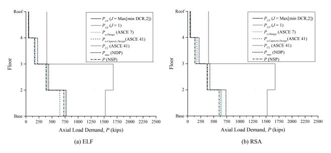
Figure 3-34. LDP Assessment Results, Compression in Exterior Columns, 4-Story EBF, BSE-2
