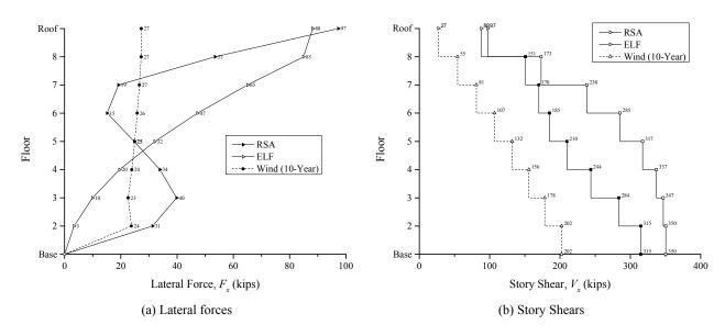
Figure B-14. Drift Design Lateral Forces and Story Shears
