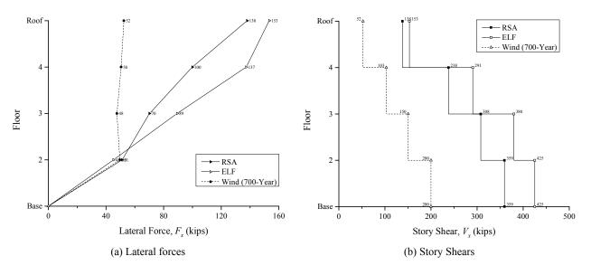
Figure B-10. Strength Design Lateral Forces and Story Shears
