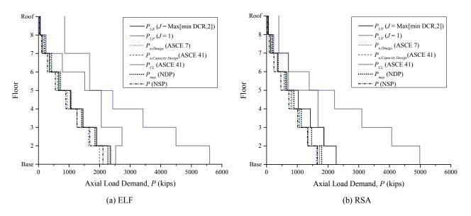
Figure 3-54. LSP Assessment Results, Compression in Exterior Columns, 8-Story EBF, BSE-1
