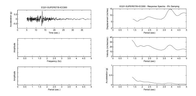
Figure A-37. 1987 Superstition Hills Earthquake at El Centro, Imperial County, Comp. 000
