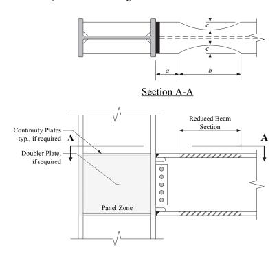
Figure 2-6. Typical Type FR RBS Beam-to-Column Connection Assembly
