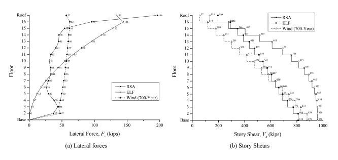
Figure B-7. Strength Design Lateral Forces and Story Shears
