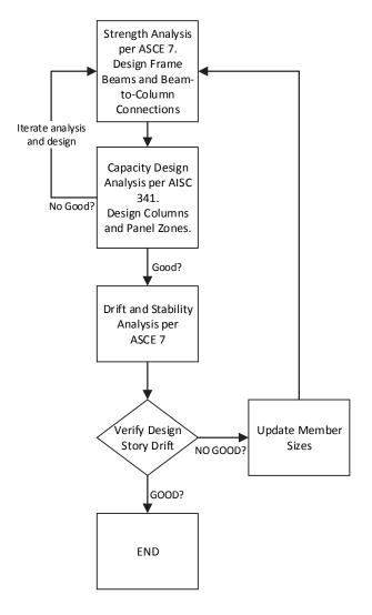
Figure 2-9. Flow Chart of SMF Design Process
