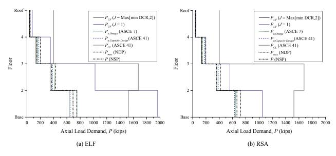
Figure 3-25. LSP Assessment Results, Compression in Exterior Columns, 4-Story EBF, BSE-1
