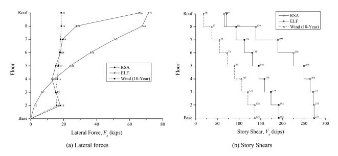
Figure B-5. Drift Design Lateral Forces and Story Shears
