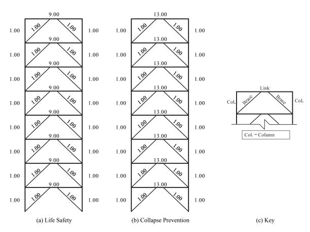
Figure 3-8. Frame Capacity Schematic (m-factor), LS and CP, 8-Story EBF ELF and RSA
