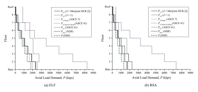
Figure 3-57. LSP Assessment Results, Compression in Exterior Columns, 8-Story EBF, BSE-2
