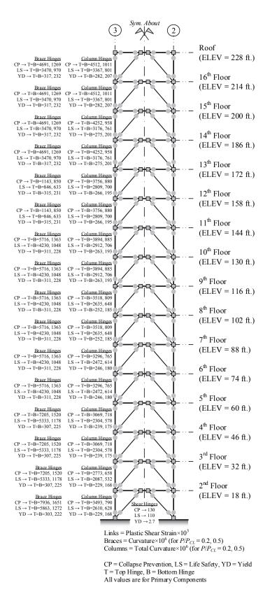
Figure 3-22. Frame Capacity Schematic (Inelastic), LS and CP, 16-Story EBF - RSA
