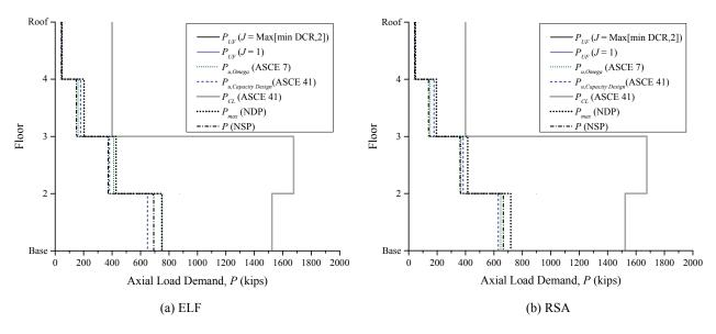
Figure 3-31. LDP Assessment Results, Compression in Exterior Columns, 4-Story EBF, BSE-1
