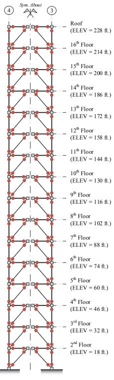
All columns, braces, and beams adjacent to link beams are *force-controlled* (FC) for flexure
