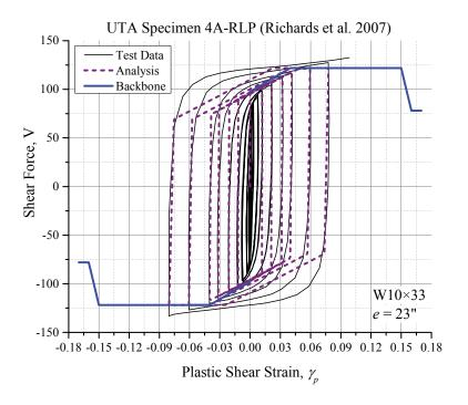
Figure 3-11. PERFORM-3D Link Beam Shear Hinge Calibration
