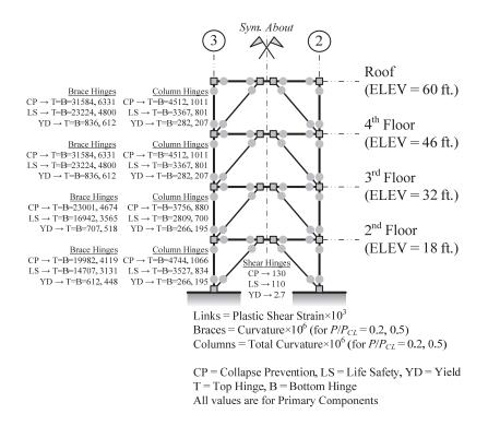
Figure 3-18. Frame Capacity Schematic (Inelastic), LS and CP, 4-Story EBF - RSA
