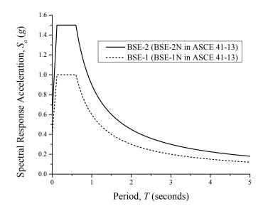
Figure 3-1. Acceleration Response Spectra
