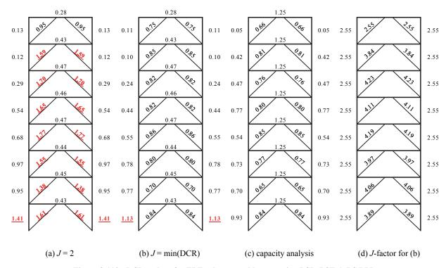
Figure 3-110. DCRN values for EBF columns and braces using LSP, BSE-1, LS BPL
