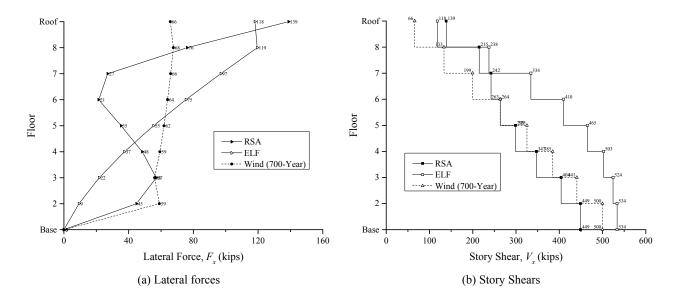
Figure B-13. Strength Design Lateral Forces and Story Shears
