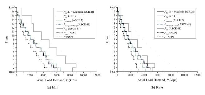
Figure 3-92. LDP Assessment Results, Compression in Exterior Columns, 16-Story EBF, BSE-2
