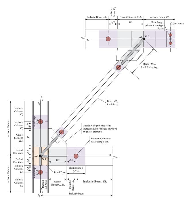
Figure 3-10. EBF Analytical Modeling Schematic
