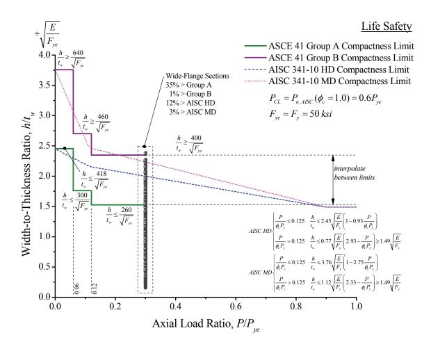
Figure 3-5. Compactness Requirements as a Function of Axial Load Ratio, LS Acceptance Criteria
