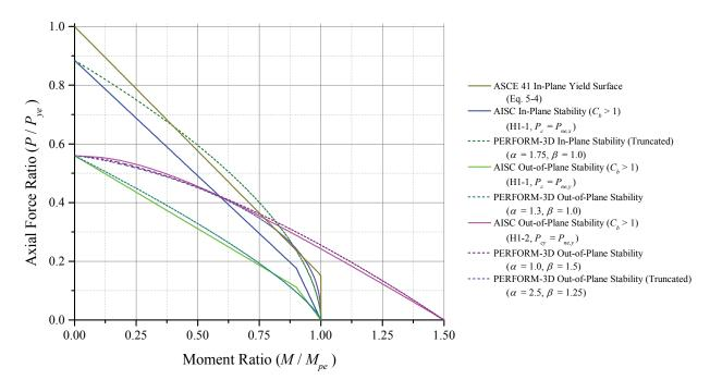
Figure 3-16. P-M Interaction Curve (Member Instability)
