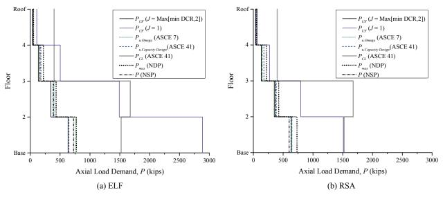
Figure 3-28. LSP Assessment Results, Compression in Exterior Columns, 4-Story EBF, BSE-2
