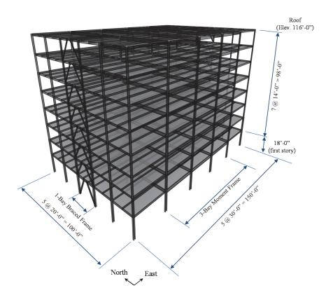
Figure 2-2. Isometric View of ME8 Archetype Building
