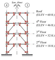
All columns, braces, and beams adjacent to link beams are force-controlled (FC) for flexure
