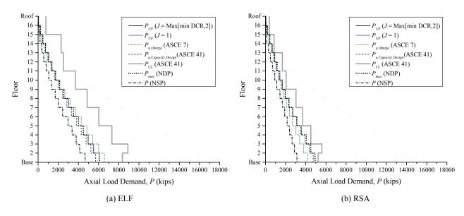
Figure 3-86. LSP Assessment Results, Compression in Exterior Columns, 16-Story EBF, BSE-2
