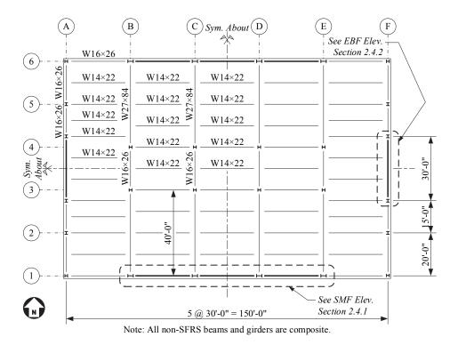
Figure 2-5. Typical Floor Framing Plan, ME16
