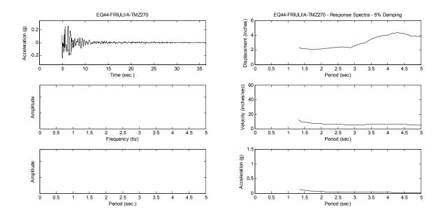
Figure A-50. 1976 Fruili, Italy Earthquake at Tolmezzo Station, Comp. 270
