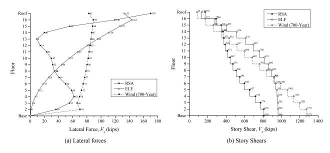
Figure B-16. Strength Design Lateral Forces and Story Shears
