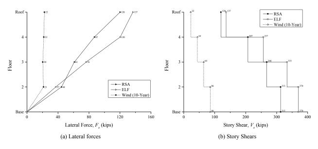
Figure B-11. Drift Design Lateral Forces and Story Shears
