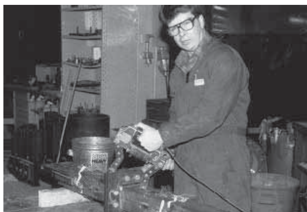
Fig. 2-4. Magnetic particle testing of an HSS connection.
