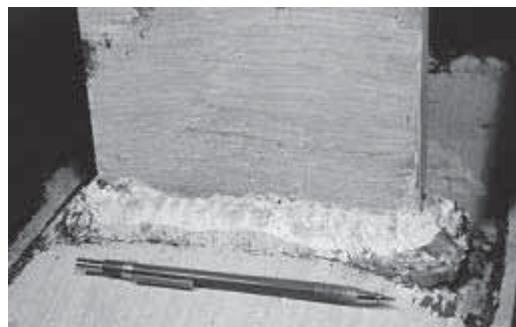
(a) Transverse plate-to-rectangular HSS connection at ultimate load. Note that rupture initiates at the plate extremities.
