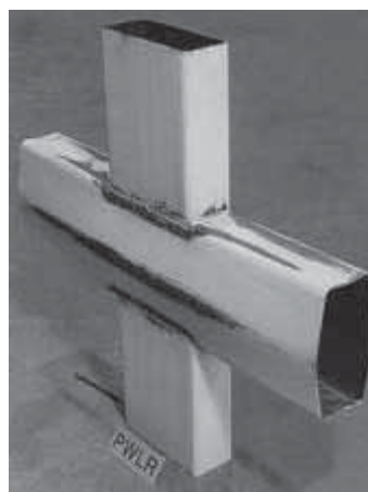
(b) Sidewall local buckling.
