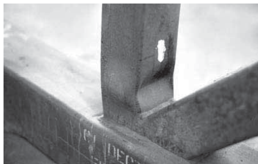
(b) Rectangular HSS overlapped K-connection at ultimate load.
